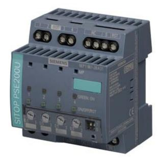
SITOP PSE200U SELECTIVITY MODULE 3A SITOP PSE200U 3 A SELECTIVITY MODULE 4 CHANNELS INPUT: 24 V DC OUTPUT: 24V DC/3 A PER CHANNEL OUTPUT CURRENT ADJUSTABLE 0.5-3 WITH STATUS MESSAGE PER CHANNEL
