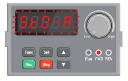
This display will flash StO-A and the motor will not start if 24V is not present on both STO channels
