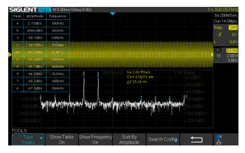
The new math co-processor enables FFT analysis of incoming signals using up to 128k samples per waveform. This provides high frequency resolution with a fast refresh rate. The FFT function also supports a variety of window functions so that it can adapt to different spectrum measurement needs. Four-channel series support Peaks, Markers, a variety of numbers.
