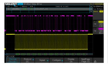
SDS1000X-U displays the decoding through the events list. Bus protocol information can be quickly and intuitively displayed in a tabular format.
