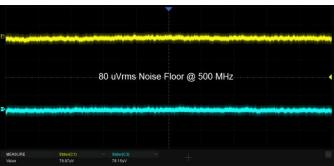
500 MHz bandwidth (at 2 GSa/s sample rate with 500 MHz Low noise floor: Only 80  $\mu$ V rms at 500 MHz bandwidth. bandwidth option).
