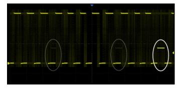
With a waveform update rate of up to 120,000 wfm/s, the oscilloscope can easily capture low-probability events. In Sequence mode the waveform capture rate can reach 500,000 wfm/s.
