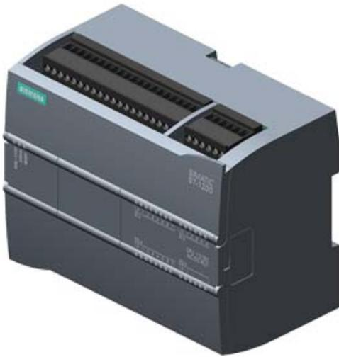
SIMATIC S7-1200, CPU 1215C, CPU COMPACTE, CA/CC/RELAIS, 2 PORTS PROFINET, ONBOARD I/O: 14 DI 24VCC; 10 DO RELAIS 2A, 2 AI 0-10V CC, 2 AO 0-20MA CC, ALIMENTATION: CA 85 - 264 V CA A 47 -63 HZ, MEMOIRE PROGR./DONNEES 100 KO
