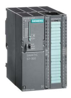
SIMATIC S7-300, CPU 313C-2 PTP CPU COMPACTE AVEC MPI, 16 E/16 S TOR, 3 COMPTEURS RAPIDES (30 KHZ), INTERFACE RS485 INTEGREE, ALIMENTATION INTEGREE 24V CC, MEMOIRE DE TRAVAIL 128 KO, CONNECT. FRONTAL (1X 40 PTS) ET MICRO-CARTE MEMOIRE NECESSAIRE
